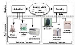
Fig. 1: High-level scheme of a building monitoring and control application.
