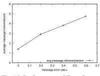
Fig. 16: Performance of TeenyLIME reliable protocol.
